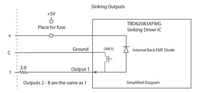
When an output is turned on, the "C" terminal is connected internally to the output terminal and provides the Ground for your external equipment.
