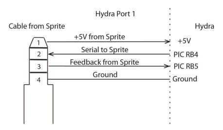
The Sprite media player connects to Port 1 of the Hydra. The Sprite will supply the 5 Volt power to the Hydra. The serial communications TX and RX are direct to the PIC processor on this port.
