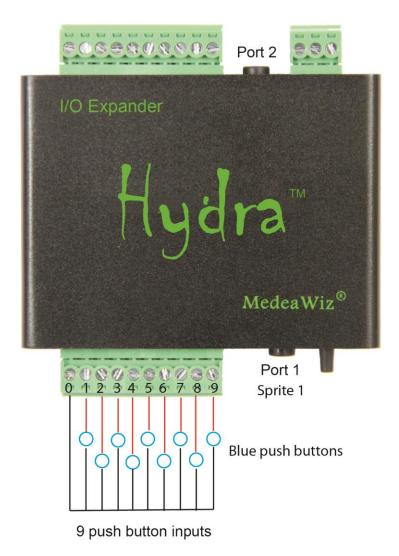
Each pushbutton should have 2 terminal connections.
