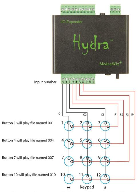
Keypads vary by manufacturer. The Columns and Rows may be in a different order than shown.
