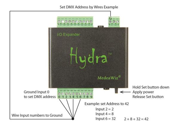
Input 0 must be grounded to let the Hydra know you want to set the DMX address . Values of any Inputs 1-9 that are grounded will add together to make the address.
