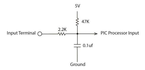
The Hydra input terminals 0 through 9 have a 2.2K series resistor to help limit current flow to a safe level for the PIC processor. There is a 47K pull-up resistor to bias the inputs to a High state. There is a 0.1uf capacitor to help reduce stray noise.
