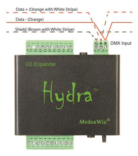
The DMX Port should only be connected to a DMX 485 bus device. Standard A, B and Ground / Shield terminals are provided. Commonly used colors are shown for Cat 5 cable above. Your colors may vary. DMX wiring for XLR and RJ45 connectors are shown below.
